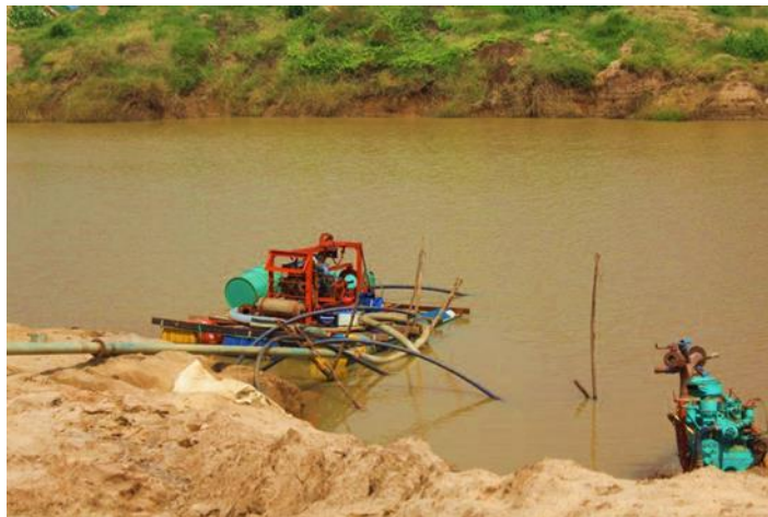
The way of sand exaction using suction pumps and machines
